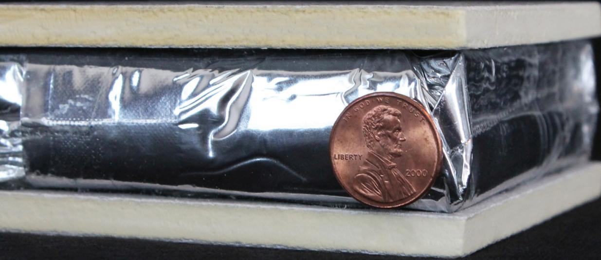
The world's only R-50 value insulation at 1.5" thickness or less.
